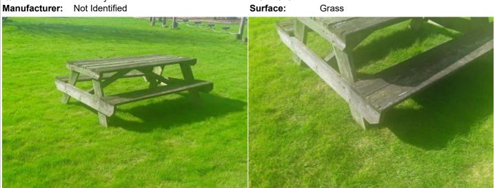
Finding: The table is not secured to the ground and there is Action: Secure the item to the ground some potential for the item to be moved within falling spaces of equipment
