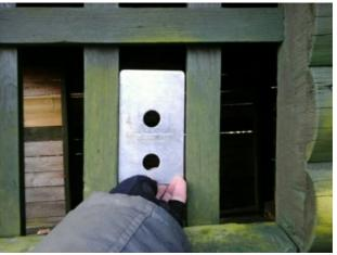
The item fails to meet the requirements of BS Action: EN 1176:2008 Part 1 4.2.7.2 for head and neck entrapment in the windows Finding: Monitor use
