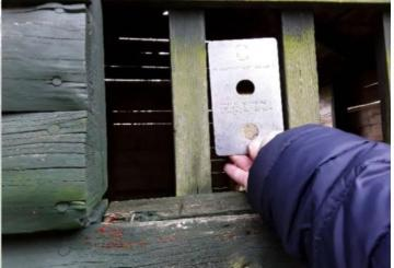
**Finding:** The item fails to meet the requirements of BS EN 1176 Part 1 4.2.7.2 for head and neck entrapment in the framework
