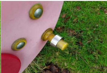
**Finding:** The end of handgrips and/or footrests have a cross **Action:** Monitor - No remedial work recommended section of less than 15cm2 and fail to meet the requirements of BS EN 1176 Part 6
