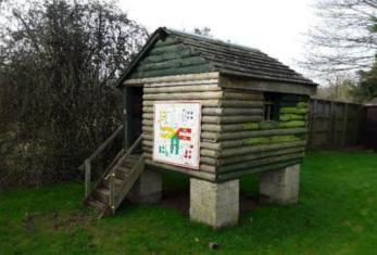
**Finding:** This equipment has not been designed or installed to meet with the requirements of BS EN 1176 for public playground equipment; we have however used our knowledge of these standards to assist in forming the basis of our risk assessment for the equipment and our report.
